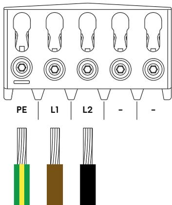
**NOTICE!** It's recommended to follow the existing colour codes used in the installation. Depending on national standards, the colours of the cables can vary from the illustrations. The illustrations in this manual follow the IEC 60446 standard.
